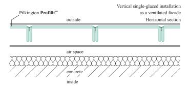
A key design element of the building envelope is Pilkington **Profilit™** profiled glass, which was installed single-glazed, ventilated cladding of the concrete walls combined with a thermally insulated composite system.
